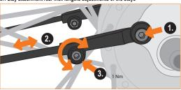
ATTENTION! Mounting of spacers for frames with disc brakes
